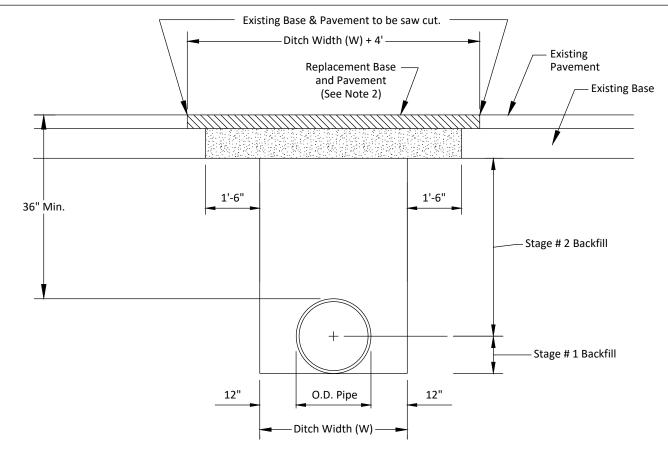
W = O.D. of pipe + 12" Min. at both sides of pipe
